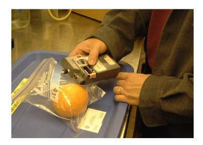
Fruit was thawed at room temperature for about 24 hours and then tested for headspace ethanol concentration. Each piece of fruit was placed in a one-quart Ziplock plastic bag for a one-hour. After equalization the bag was sampled for ethanol with an Alcosensor IV (Intoximeters, Kansas City, MO). The sensor was factory modified with a hypodermic needle probe allowing the bag to be sampled. Fruit was then manually evaluated for freeze damage using the USDA procedure for recently frozen oranges.
