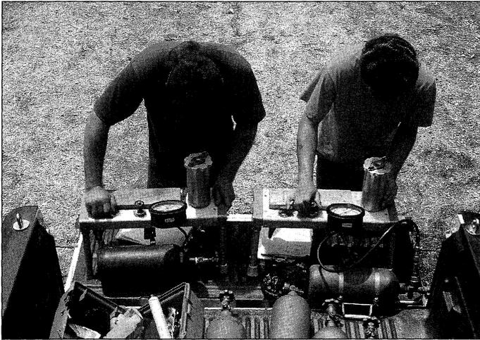
Technicians use pressure chambers to simultaneously measure leaf and stem water potential; both indicators of tree water stress.
